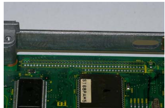
Pads de-soldered for Adaptor B
