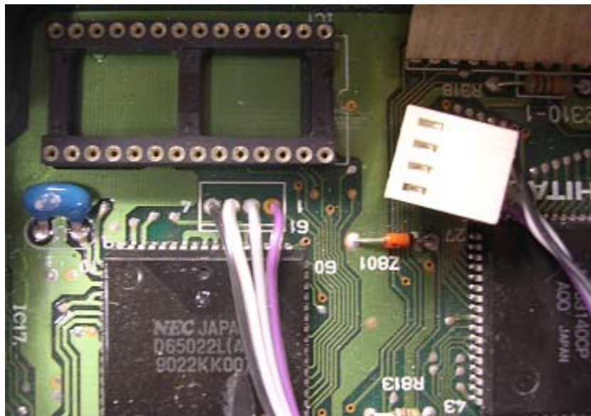
BNR32 CPU cable installation
